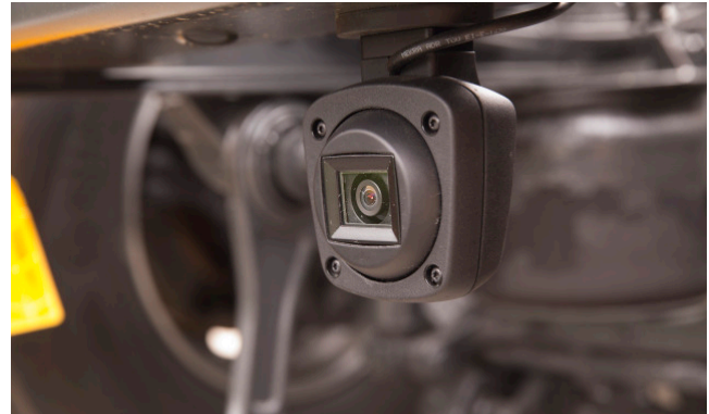
Panoramic view for the driver: The SurroundView system can cover the side of the vehicle as well. Up to four cameras can be connected to the monitor.
